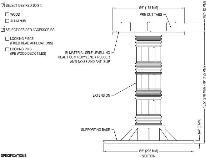
MATERIAL: POLYPROPYLENE AND RUBBER (HEAD TOP FINISHING) [RECYCLABLE MATERIAL]
